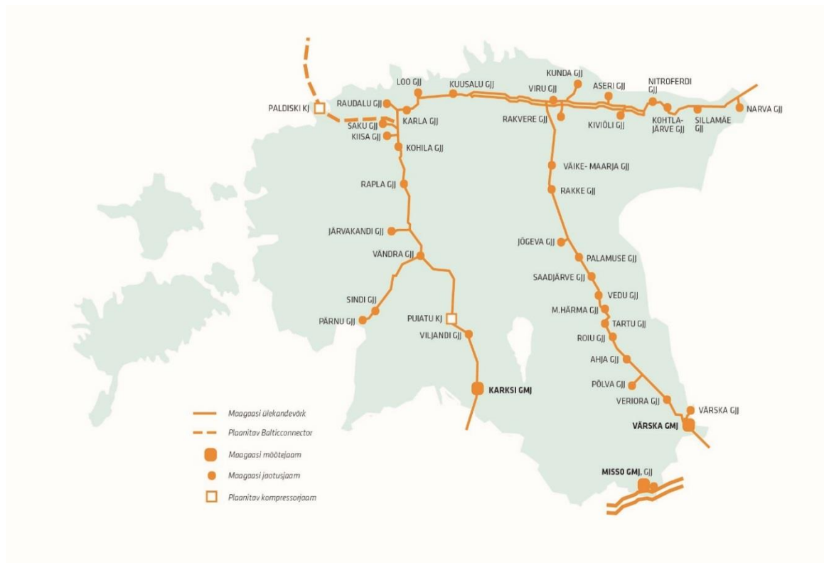
Figure 1. Estonian natural gas transmission network
