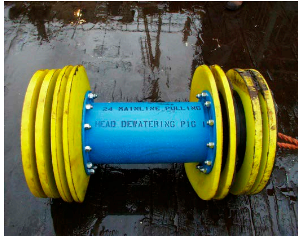
Figure 3-20. A typical de-watering pig (Ramboll 2014a).
