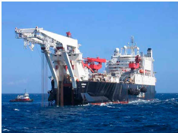
Figure 3-12. Typical pipelaying vessels - a dynamically positioned pipelaying vessel ( Solitaire , left) and anchored pipelaying vessel ( Castoro Sei , right) (Ramboll 2013).
