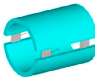
Figure 3-3. Example of an aluminum bracelet anode (Ramboll 2014).
