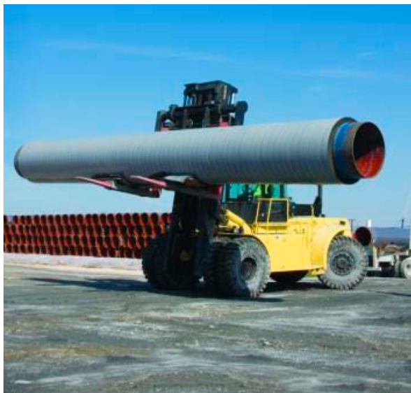
Figure 3-2. Line pipe with a (black) polyethylene coating inside a concrete coating (Ramboll 2014c).
