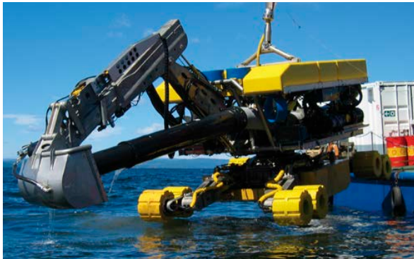
Figure 3-6. Dredging techniques. Shown left is a remotely operated “spider” and right a dredging barge and loading vessel (Ramboll 2014a).
