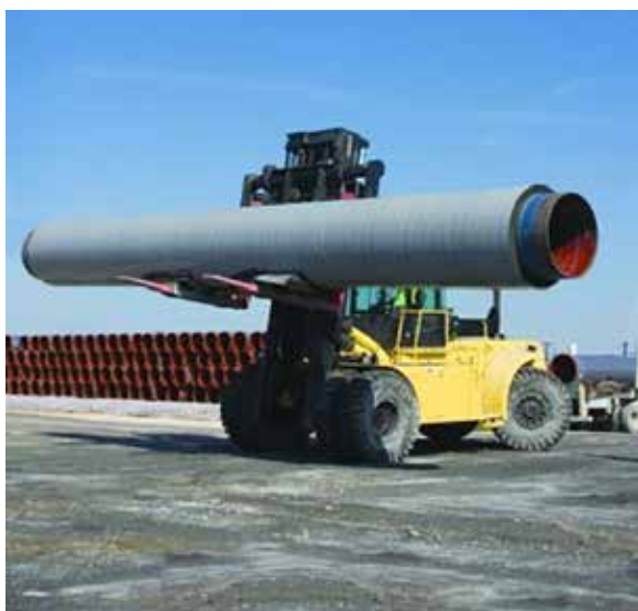
Figure 1.15. Pipe joint provided with PE coating (black) underneath the concrete weight coating
