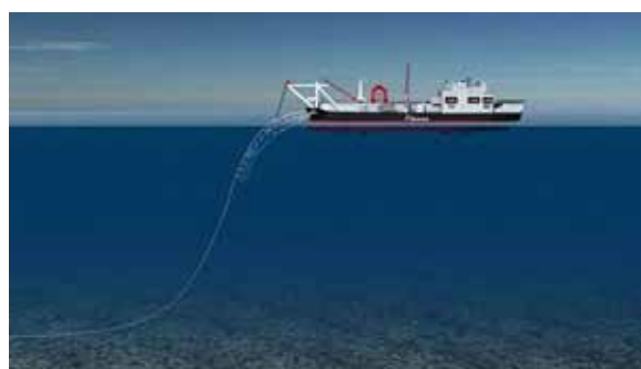
Figure 1.12. S-lay with DP pipelay vessel (Allseas.com, 2013)
