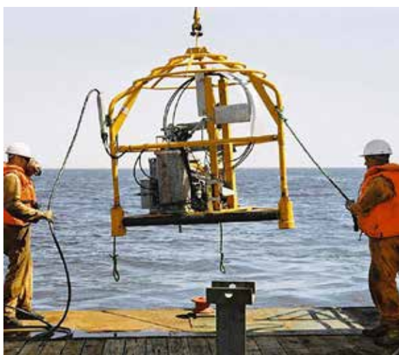
Figure 8.1. A typical cone penetration rig. Among other sampling, the seabed survey will include cone penetration testing to study the geotechnical features of the seabed.
