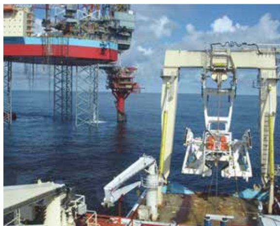
Figure 1.13. Typical trenching spreads - During launching with A-frame and on deck
