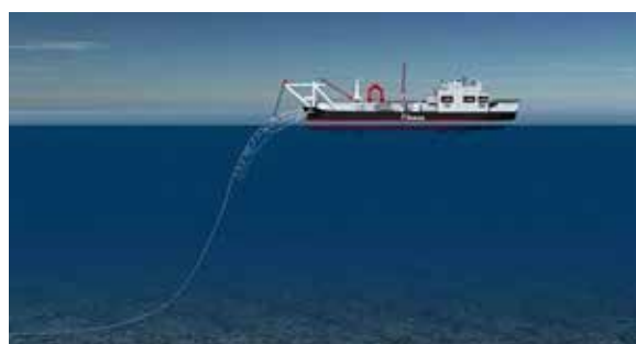
Figure 2. S-lay with DP pipelay vessel (Allseas.com, 2013)
