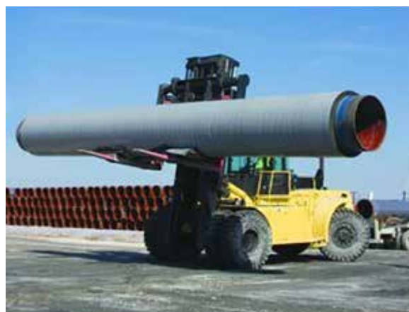
Figure 3. Pipe joint provide with PE coating (black) outneath the concrete weight coating
