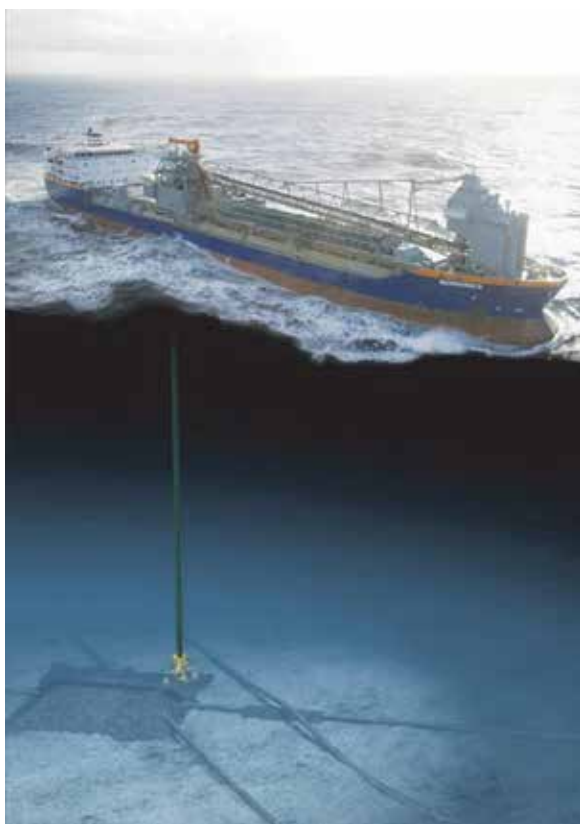
Figure 1.17. Rock installation using specialized fall pipe vessel
