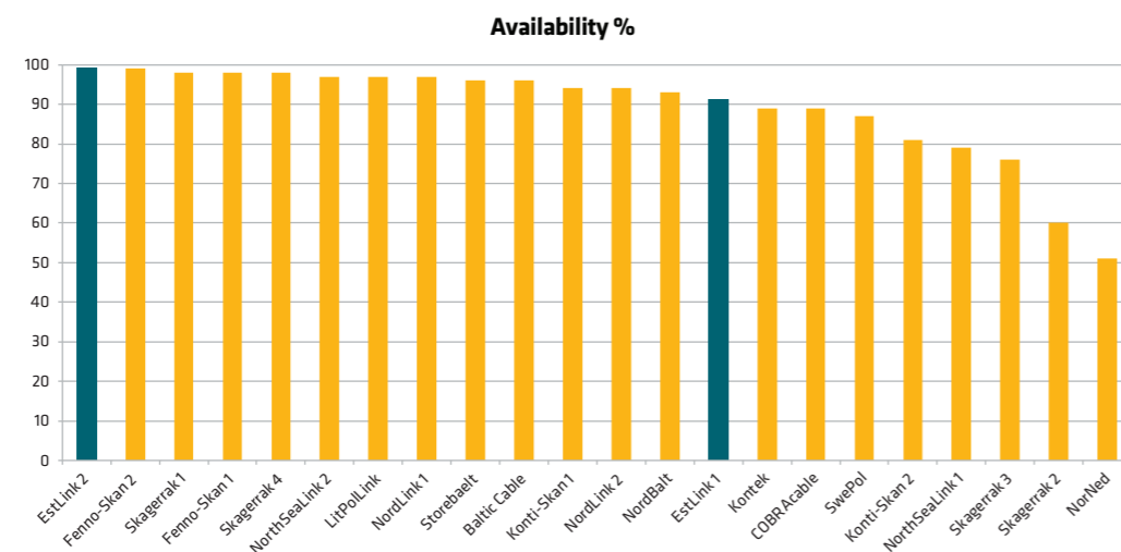
Figure 2.14 Percentage of the capacity of availability of Nordic and Baltic direct current cables in 2022
