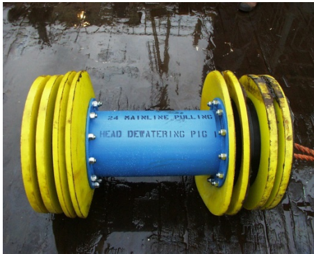
Figure II-2 Typical de-watering pig
