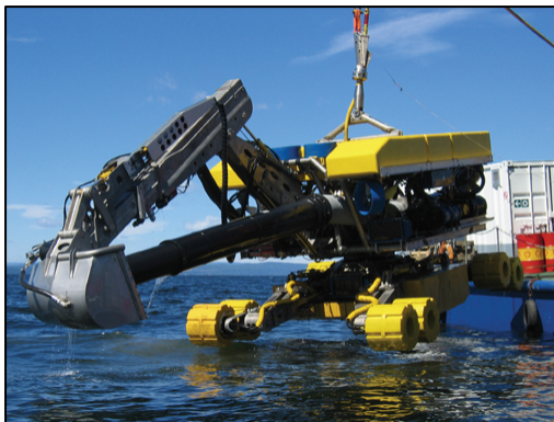
Figure 11-3 Dredging techniques using spider (left) and dredging barge and cargo vessel (right)
