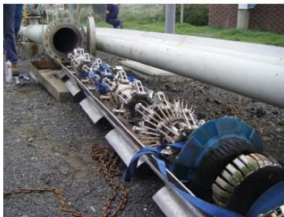
Joonis 6-26A. Torustiku sond (pig) (viide: Koh, J. Analysis of the noise and vibration in the pipe near PIG Launcher, Korea Gas Corporation)
