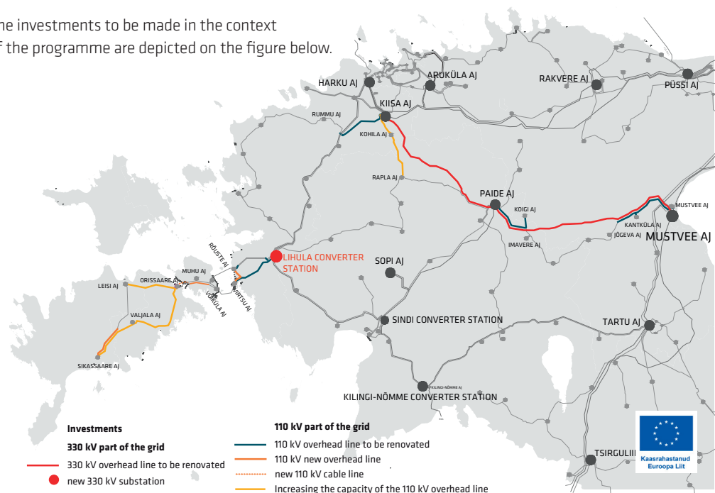
Figure 3.5 Investments that allow increasing the capacity of the western Estonian and islands' dispersed and renewable power grid
